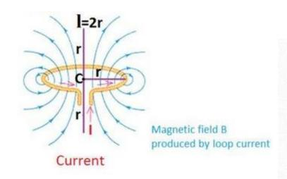
The magnitude of the magnetic field at the center of a circular loop with a radius R and carrying current I is
